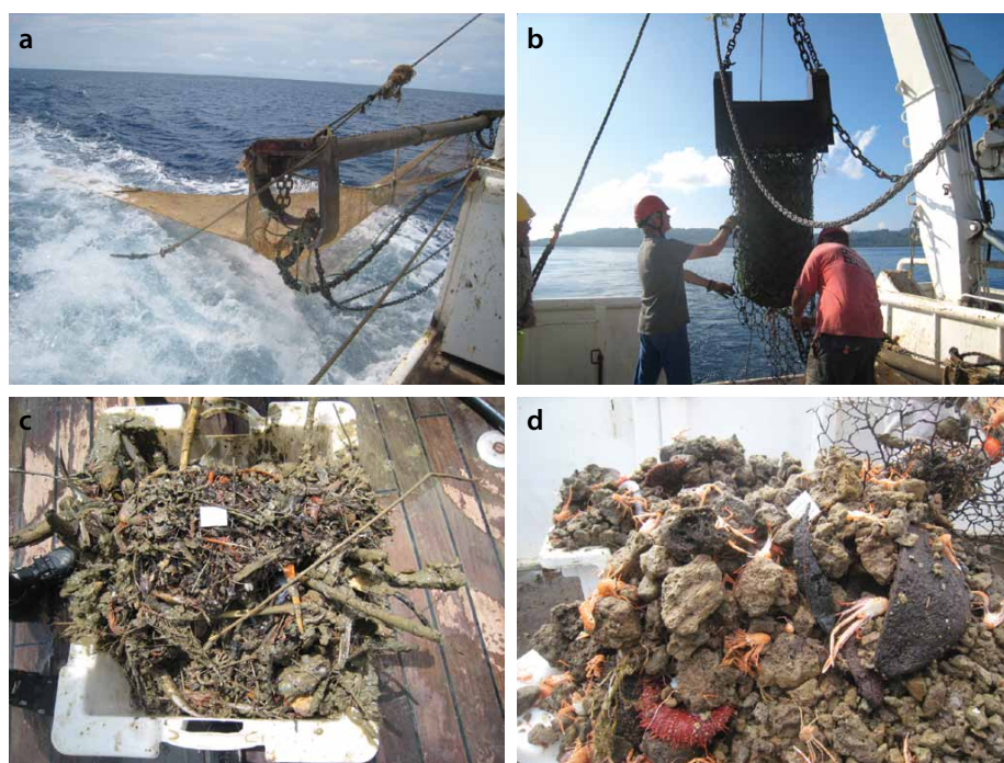
Figure 3. Sampling strategy employed during BioPapua and other Tropical Deep-Sea Benthos cruises. (a) Beam trawl. (b) Warén dredge. (c–d) Raw samples that illustrate the abundance of fauna collected and the diversity of substrates.
