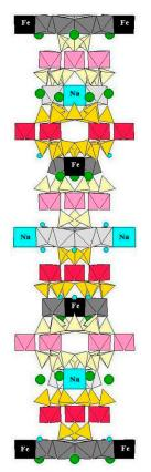
Figure 11. Alternation of Na- and Fe-centered squares in rastsvetaevite [49,50].
