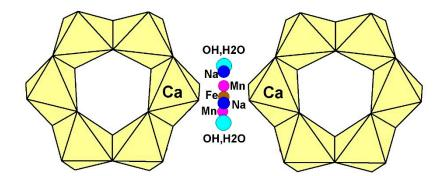
Figure 4. Cation distribution over M2 sites between CaO<sub>6</sub> octahedra in Sample 4 (Table 4) [29].
