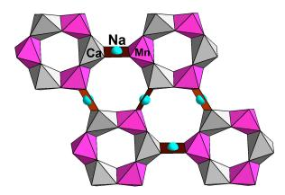
**Figure 6.** Combination of the rings of Ca- and Mn-centered octahedra via Na atoms having flat square coordination in the structure of Sample 10 (Table 4) [30].
