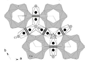
Figure 9. Seven-vertex M2 polyhedra in Sample 3 (Table 4) [32].
