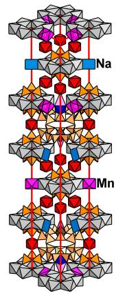
**Figure 10.** Alternation of Na- and Mn-centered square pyramids in the Mn-rich, alluaivite-type Sample 22 (Table 4) [51].
