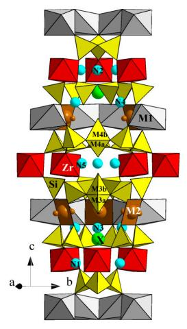
Figure 1. The crystal structure of eudialyte-group minerals (a simplified sketch).
