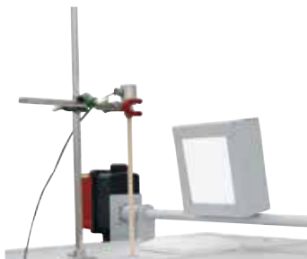
Exhaust air flap and charge thermocouple including a stand as additional equipment
