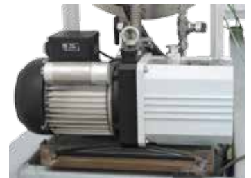
Vacuum pump for cold evacuation of the retort
