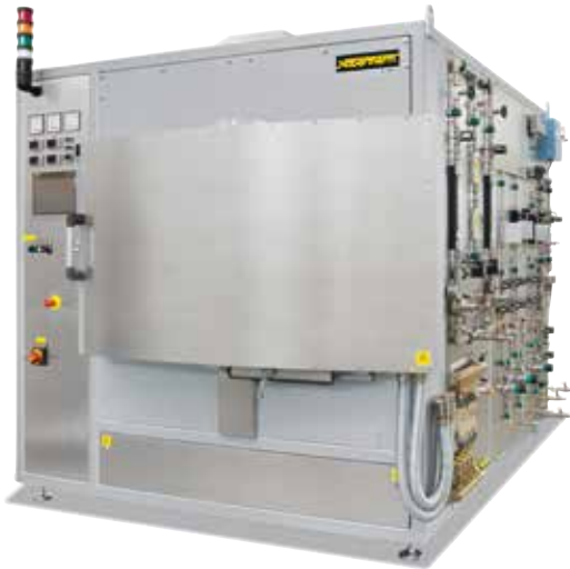
NRA 300/09 H 2 for heat treatment under hydrogen
