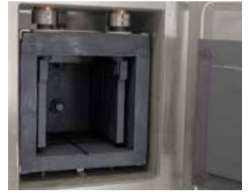
Graphite heating chamber
