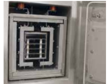
Molybdenum heating chamber
