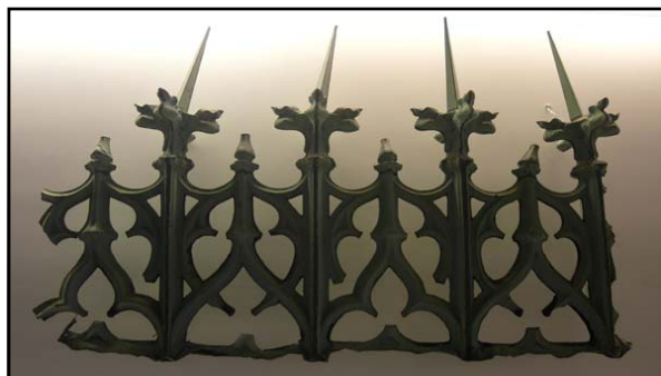
Above: original copper tracery. The gabled roof/s and 30th Floor setback/s of the main office block (base) were decorated with delicate filigree made of hollow copper. It was removed due to deterioration caused by acid rain. 749
