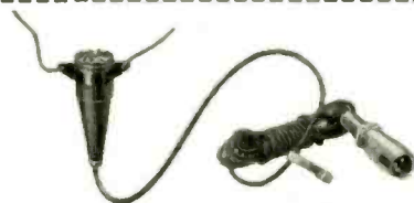
ALTEC 686A LAVALIER MICROPHONE Frequency Response: 70 to 20,000 cycles • Output Impedance: 30/50, 150/250 ohms • Output Level: -55 dbm/10 dynes/cm 2 • Hum: -120 db (Ref.: 10 -3 Gauss) Price: $45.00 net
