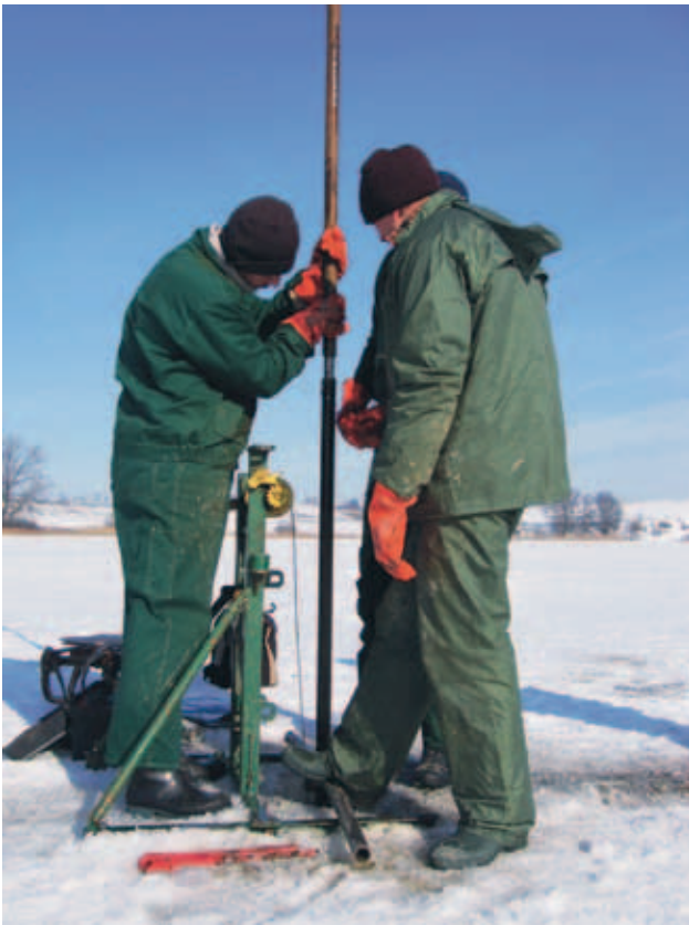
Fig. 5. Drilling by the Wieckowski probe from the ice surface. Photo: Marta Szal
