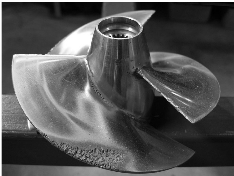
Figure 10: Cavitation damage evident on the propeller of a personal watercraft.
