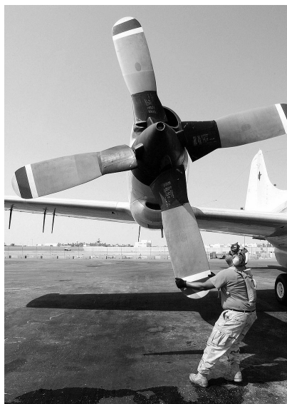
Figure 2: Rotating the Hamilton Standard 54H60 propeller on a US Navy EP-3E Orion's number four engine as part of pre-flight checks
