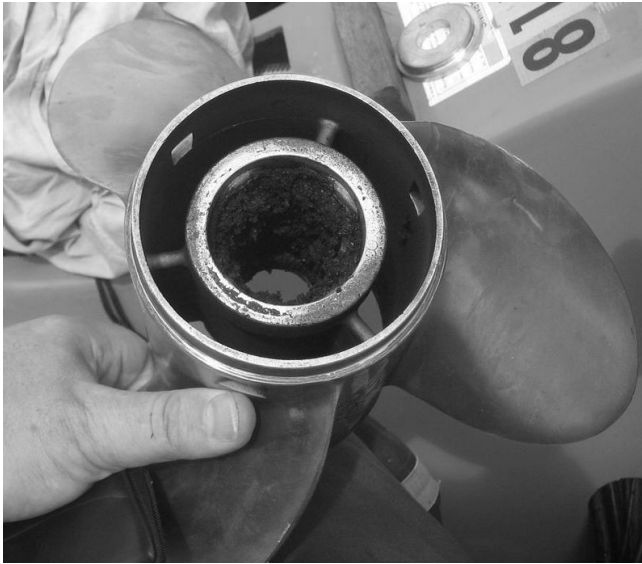
Figure 13: A failed rubber bush in an outboard's propeller
