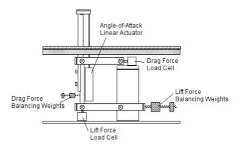
Figure 4: Diagram of Force Balance.
