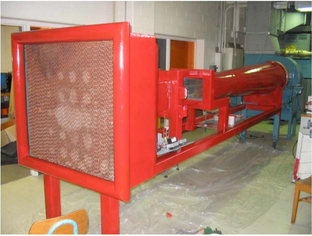
Figure 3: Picture of subsonic wind tunnel upgraded in this work.
