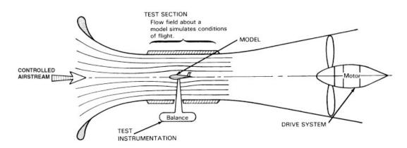
Figure 2: Diagram of typical wind tunnel.
