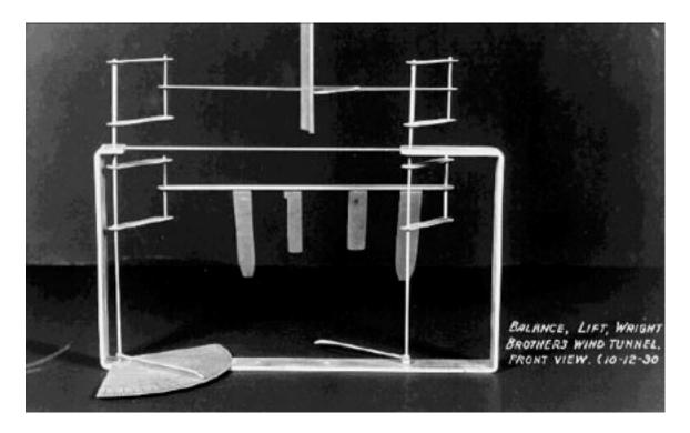
Figure 1: Force balance used in Wright Brothers' wind tunnel.
