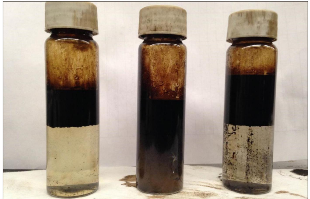
Figure 5 From left to right: an emulsion treated with caustic, no chemistry, and a standard emulsion breaker
