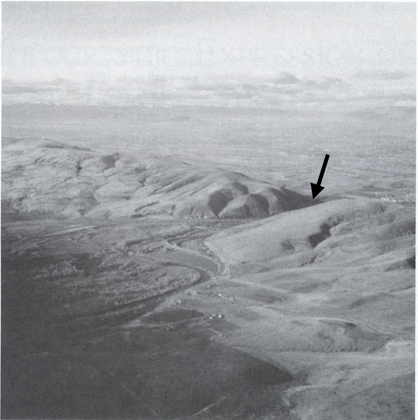
FIGURE 9-1 Anticlinal ridge cut by an antecedent stream, the Yakima River, cutting across Umtanum Ridge, Washington.
