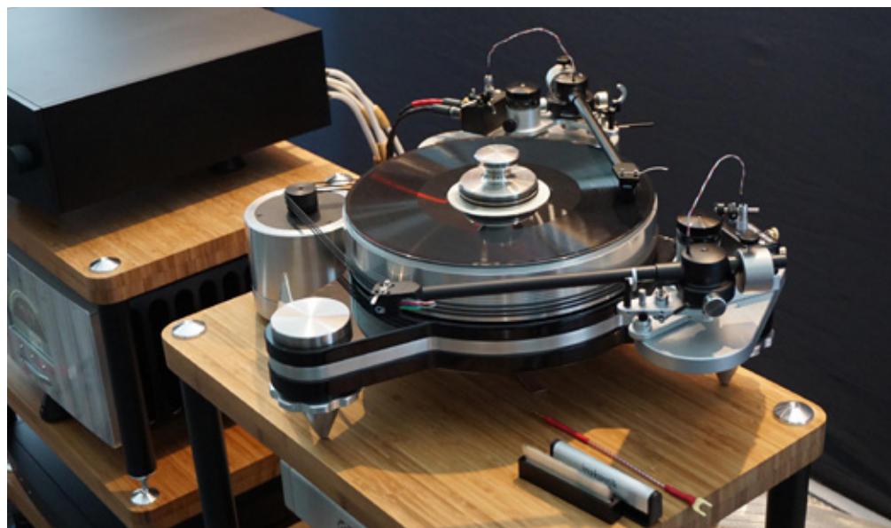
VPI's new belt-driven Avenger turntable uses multiple drive belts to share the platter-spinning workload
