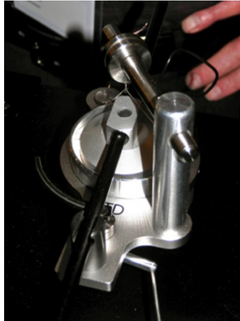
Well Tempered's Symmetrix LTD tonearm uses a thread-type bearing, as this close-up reveals
