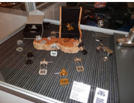
The Arche tonearm headshell from Acoustical Systems offers special provisions for adjusting azimuth, stylus rake, cartridge overhang and alignment
