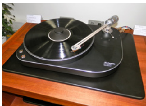
The Swiss-made Thales Simplicity is a fine example of a tangential-tracking tone arm. Note how a control arm allows continuous, on-the-fly adjustment of cartridge alignment via the tonearm's articulated, pivoting headshell
