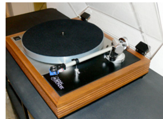
The classic Linn Sondek LP-12 turntable is a suspended chassis design that has continued to evolve from the 1970s to the present day (the sample shown is from the mid-1980s and is still in use today)
