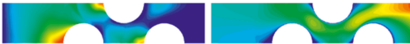
Figure: Pressure (left) and normal velocity (right) fields in a left-to-right granular flow around obstacles
