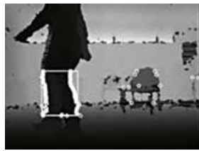
Qbo robot with laser-sensor leg detection
