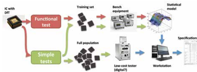
Fig. 1 Machine learning based production test of integrated circuits.
