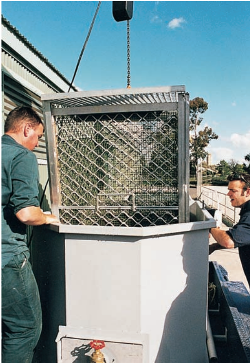
Trap-and-truck fishways allow carp to be removed and native fish to be placed upstream of dams and weirs. Source: A. Toovey, NSW Fisheries.
