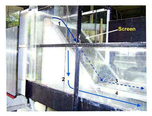
Figure 2: Two dimensional model trial of Coanda screen.
