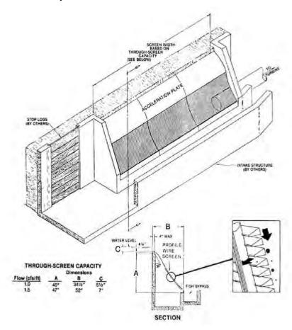
Figure 1: Schematic of Coanda screen.
