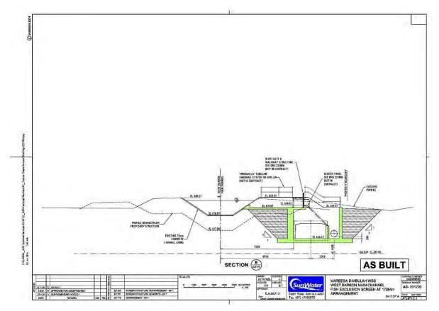
Figure 4: Cross section of the West Barron Main Channel fish exclusion screen
