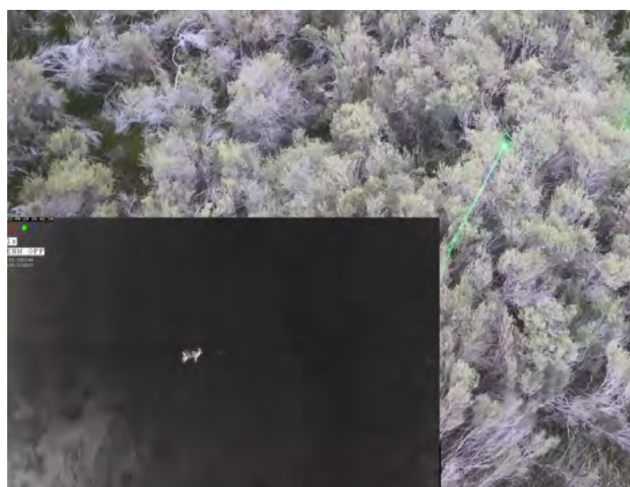
Figure 10. Thermal video cameras fitted to helicopters or drones can clearly and quickly detect feral deer in dense vegetation (bottom left), compared with the ability of the human eye (colour image). Photo from HeliSurveys.
