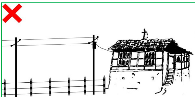
Figure 3A. Electric fence in parallel with power line
