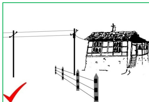
Figure 3B. Electric fence line in perpendicular to power line
