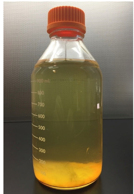
Saturated oryzalin solution in a clear bottle to demonstrate precipitation. Photo courtesy of Bob Hamilton.
