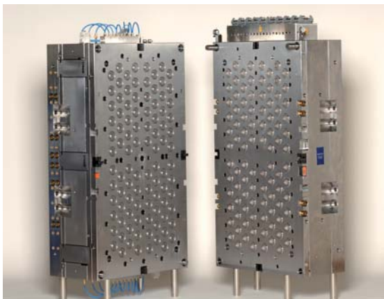
The 96 cavity mould tool cycles at 3s for the 1g cap
