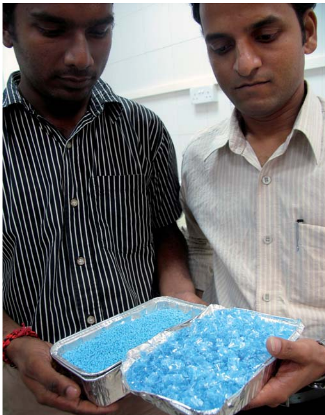
Vinod M. Shetye and Dinesh Cranonkar show the products at the recycling plant. In the foreground the light blue washed and sorted flakes from post-consumer bottles and behind is the PET granulate, also tinted light blue.
