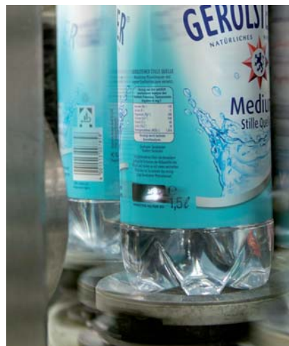
The laser beam thermally alters the outer surface of the product.
