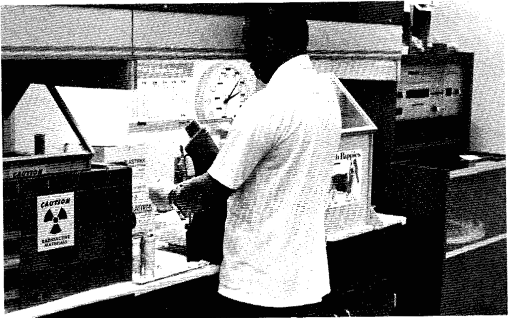
Fig. 1-4. Dose of radiopharmaceutical is withdrawn from vial in lead container into syringe. Radiopharmacist works behind lead shield and observes work through leaded glass window shield.
