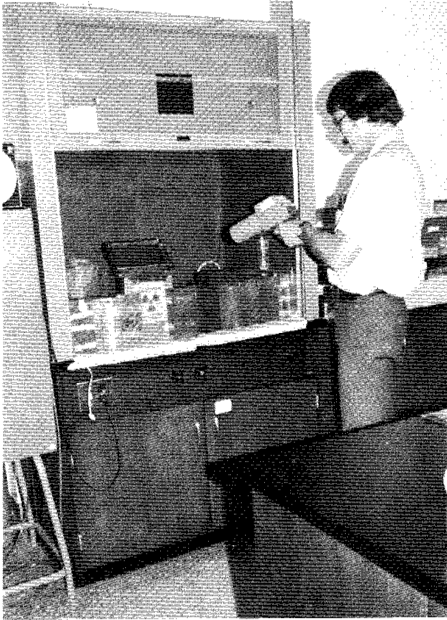
Fig. A-9. Lead-shielded areas enclosed in a fume hood used for dispensing of volatile radiopharmaceuticals such as iodide 131 solution and xenon 133 gas. In foreground is radiation safety officer monitoring background levels in radioisotope hood.
