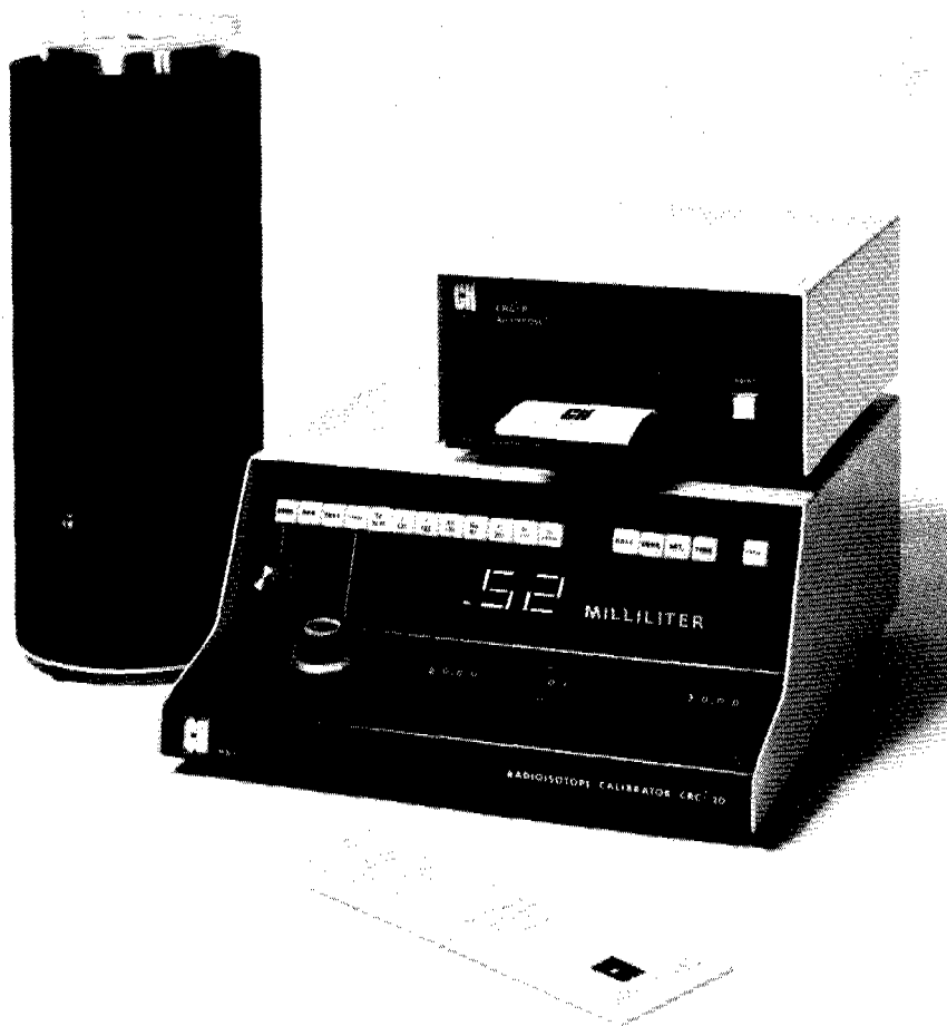
Fig. 11-3. Radiation dose calibrator. (Courtesy Capintec, Inc.)
