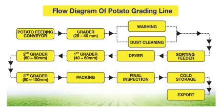
Figure 82 Potato Grading Line Courtesy: IAC
