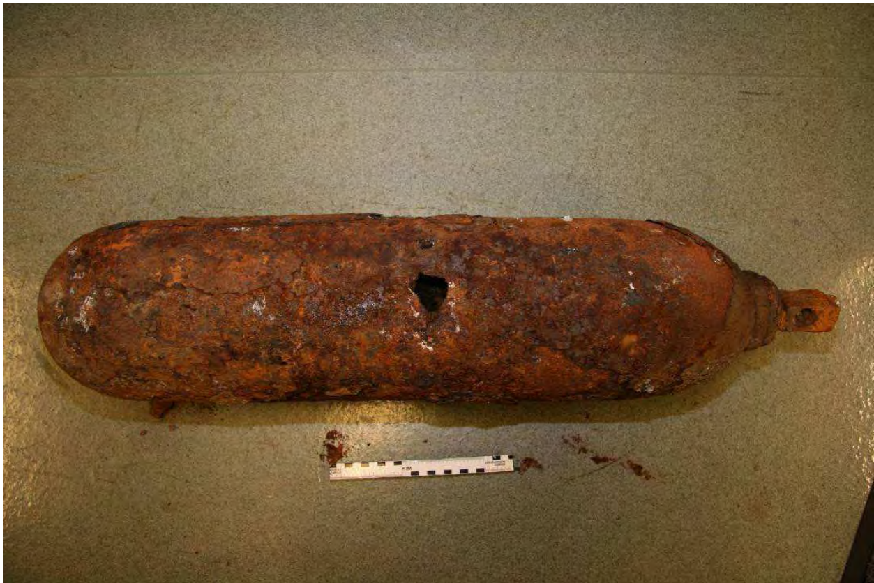
Figure 5-1 Steel canister for pressurised air (diameter 200 mm)
