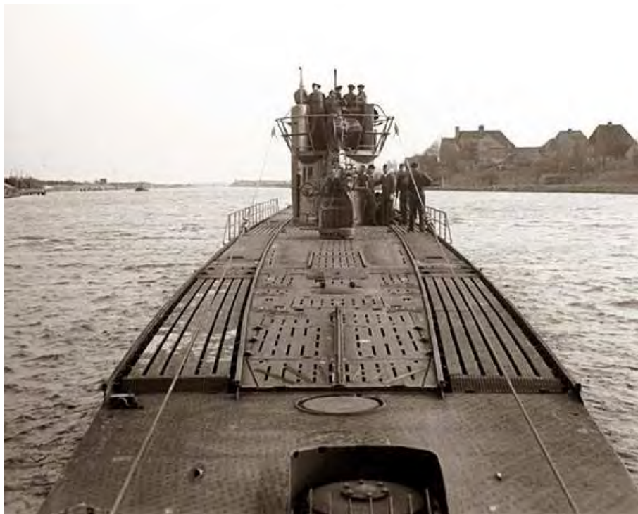
Figure 8-3 The after deck of U-166, a type IX C submarine (similar to U-864, but approximately 11 metres shorter) /7/. This picture shows the wooden trapdoors on each side which torpedoes are stored beneath. A total of 12 torpedoes is expected to have been stored like this on U-864.
