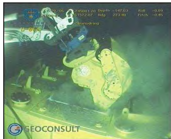
Figure 4-3 Excavator equipped with a visor bucket (system developed by Scannudring and used for dredging to reach the keel of U-864 in 2006)
