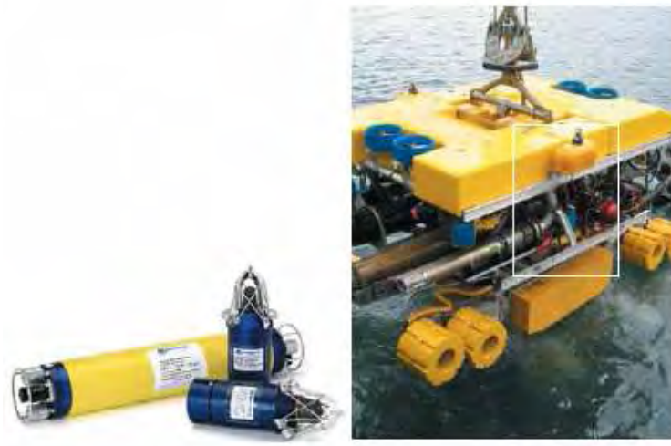
Figure 5-3. Typical ROV mounted equipment for LBL positioning (/12/)
