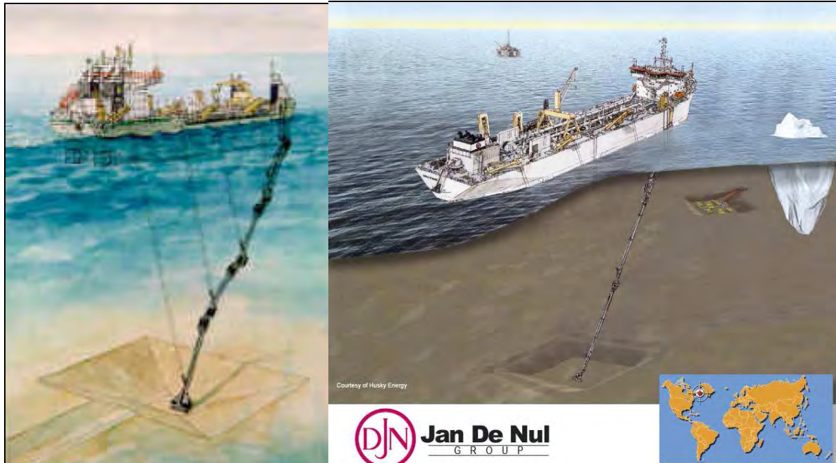
Figure 4-5 Left: Dredging down to 106 m water depth (from Glory Holes project, Canada /3/. Right: Dredging down to 130 m depth (continuation of Glory Holes project, Canada /4/,
