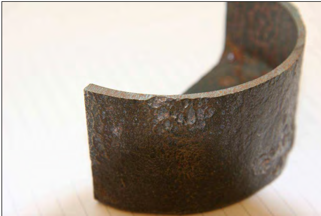
Figure A-1 Segment cut from bottom forged mercury container (diameter 140 mm) through area with maximum metal loss. (All external surfaces have been grit blasted)
