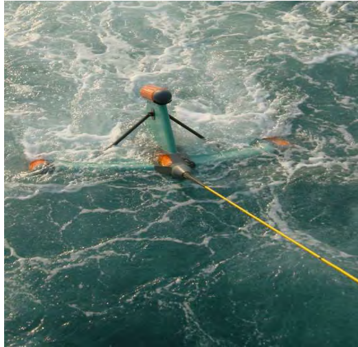
Figure 4-8. The three-axis gradiometer system. (/13/, /8/)
