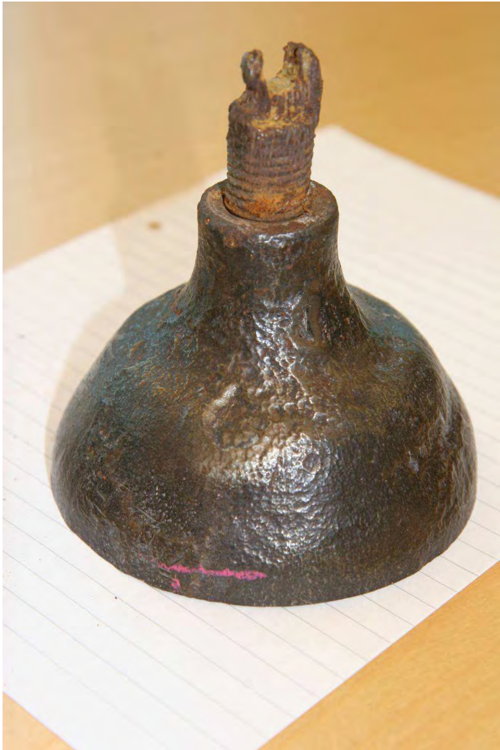
Figure A-3 Top section of forged container for mercury
