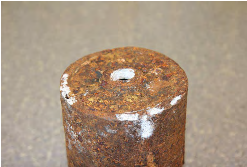
Figure A-5 Top section of welded mercury container (Leak area at the periphery to the left)
