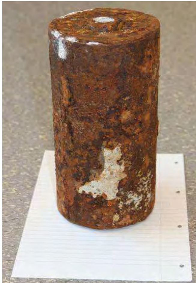
Figure 5-4 Welded mercury canister (diameter 130 mm)
