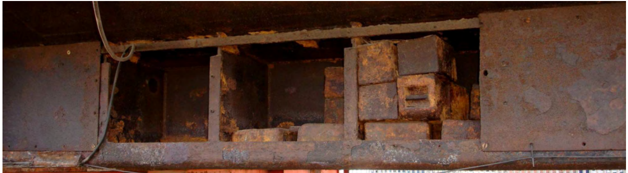
Figure 5-2 The storage room in the keel of U-534 (Type IX C, similar to U-864 but approximately 11 metres shorter)
