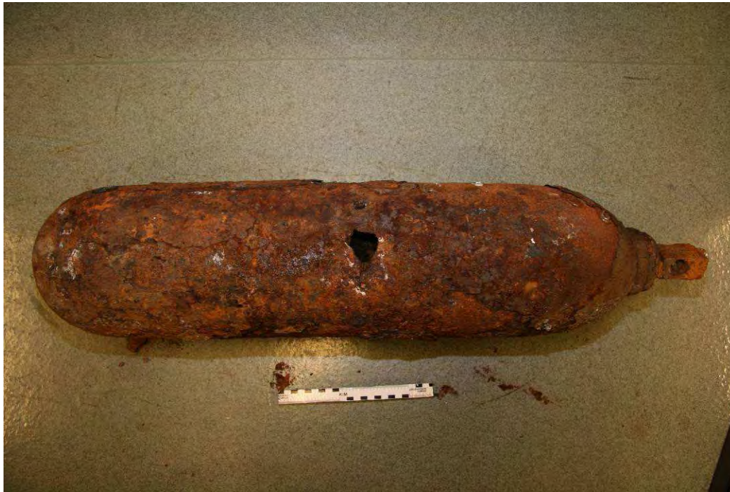
Figure A-7 Steel cylinder for pressurised gas (diameter 200 mm)
