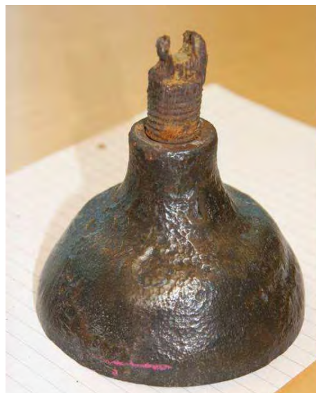
Figure 5-3 Top section of forged container for mercury
