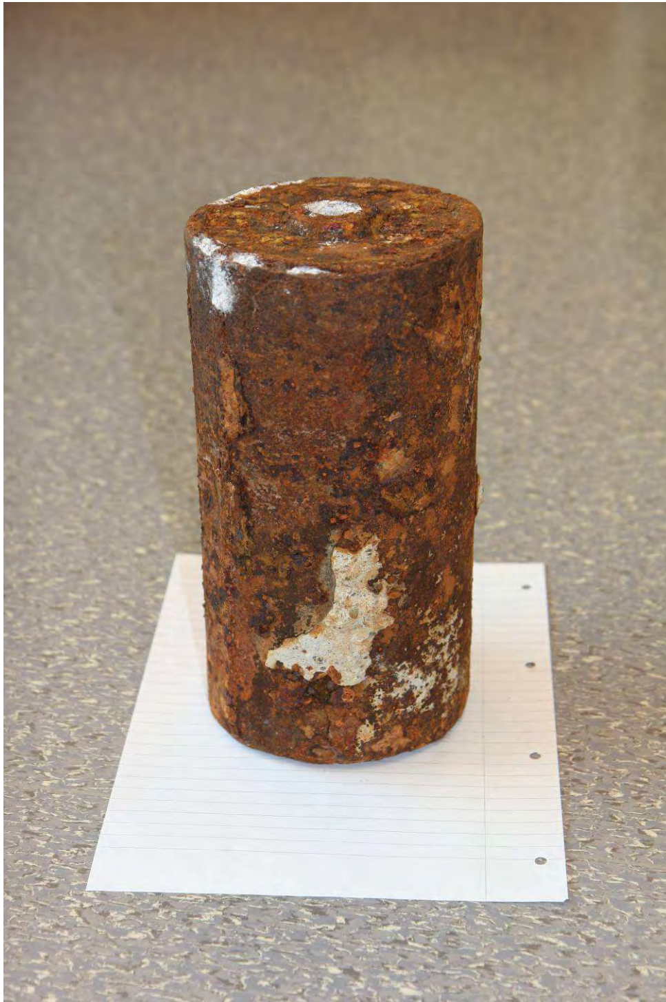
Figure A-4 Welded mercury container (diameter 130 mm)
