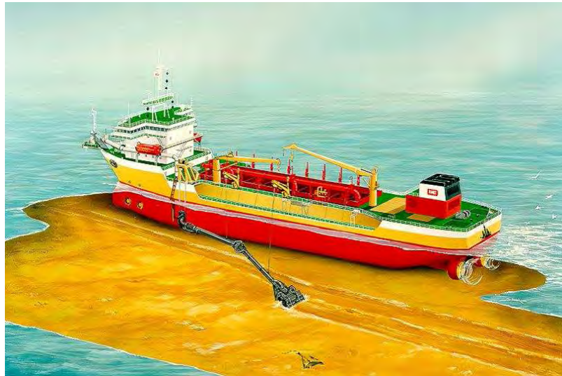
Figure 4-4 Trailing suction hopper dredge (TSHD)
