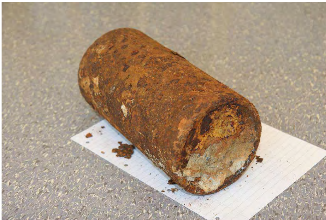
Figure A-6 Bottom section of welded mercury container
