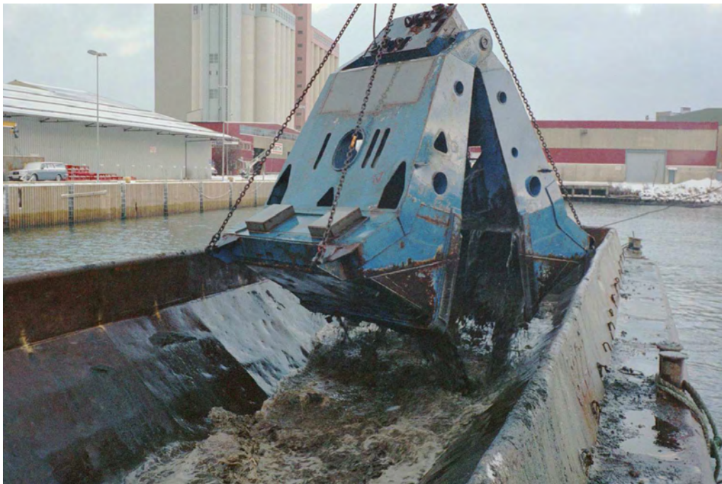
Figure 4-7 Closed level cut clamshell (photo from environmental dredging works in Trondheim harbour, Norway)
