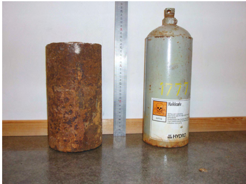
Figure 4-1. Original and modern mercury canisters
