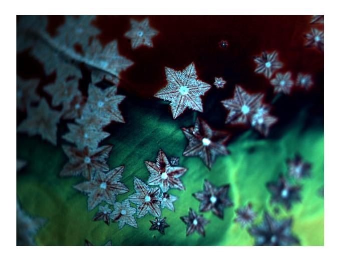
Snowflakes etched in graphene at Skoltech. The light areas are graphene, and the dark ones are oxidized copper. The snowflake pattern emerged as the surrounding graphene was etched away by carbon dioxide in one of the experiments before the optimal gas composition was found. Credit: Artem Grebenko/Skoltech
