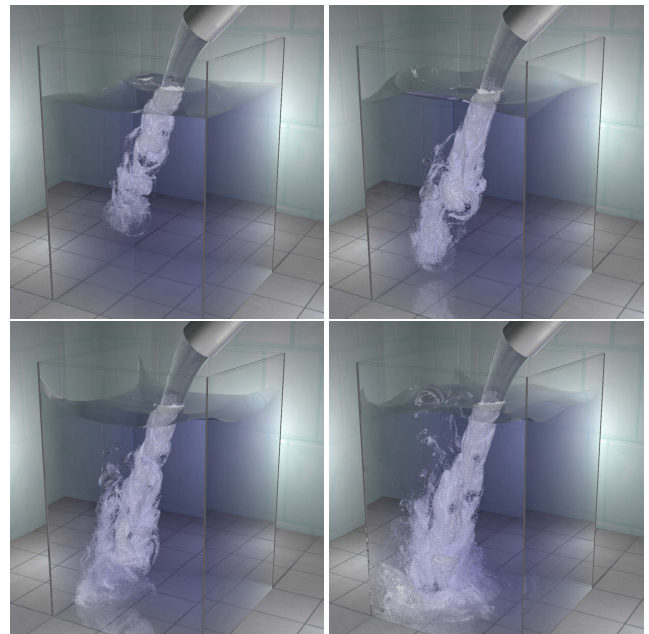
Figure 10: Faucet pouring water showing air entrainment ( 200 \times 400 \times 200 grid in a 1m \times 2m \times 1m domain); about 300,000 sub-grid bubbles. Note that the size of the sub-grid bubbles was accentuated to highlight the complex bubble interactions and the dynamic flow field.
