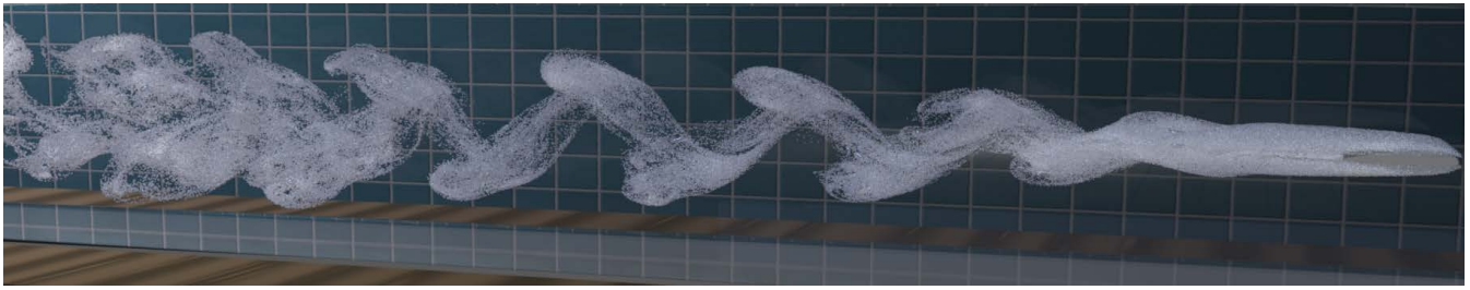
Figure 7: A fast moving hydrofoil generates the typical Von Karman vortex street in its wake through cavitation. The vortex street is generated because of the two-dimensional cross-sectional nature of the hydrofoil ( 1024 \times 128 \times 128 grid in a 50m \times 200m \times 50m domain); about 600,000 sub-grid bubbles.
