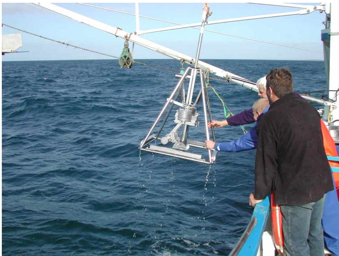
Figure 2.2. HAPS corer being retrieved after collection of sediment sample (photo S. Madigan).
