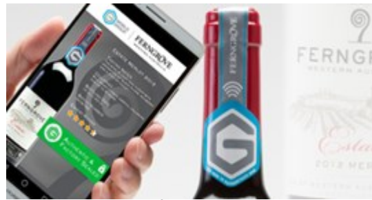
Figure 8. Commercialised intelligent RFID- based packaging system for wine (Thinfilm, 2015 b, Thinfilm, 2015c). Photo courtesy of Thin Film Electronics ASA.
