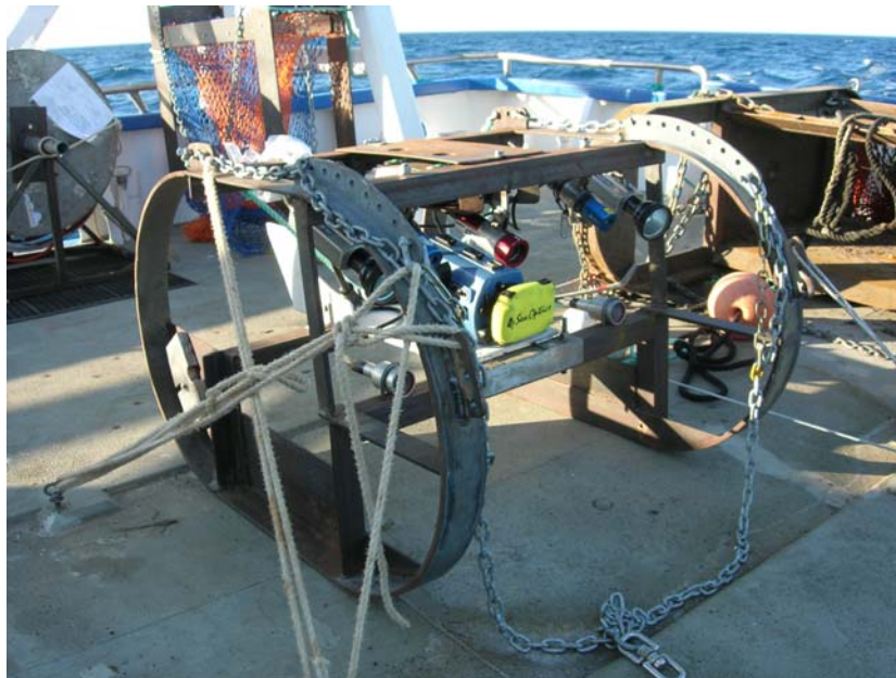
Figure 4. Underwater camera system used to quantify epibenthos and seafloor topography at 11 sampling sites inside the BPZ during October 2006.
