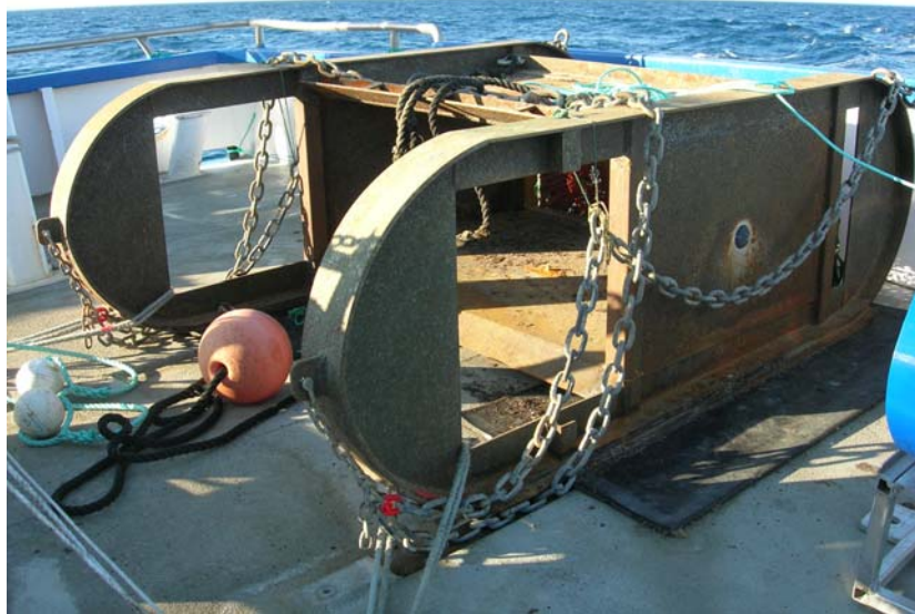
Figure 3. Epibenthic sled used to collect sessile organisms from 40 sampling sites inside and immediately outside the BPZ during October 2006.
