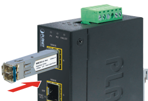
Figure 2-3: Plug-in the SFP Transceiver
