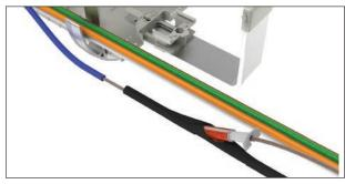
If needed, the Wire Loom Insertion Tool (Catalog Number: 80813518) can be used to install the split braided wrap onto the bare fibers/ribbons.
