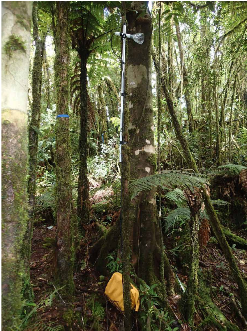
Figure 6.1. Set up of the D500X bat detectors. The microphone is placed in a funnel and tied to a pole 2.5 m from the ground, and the detector is placed inside a waterproof bag.
