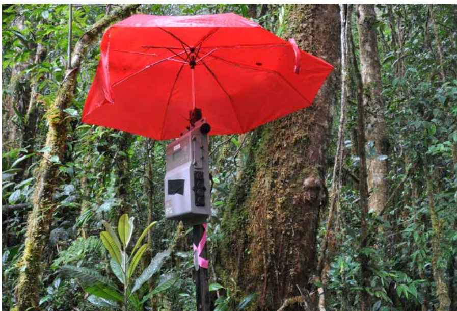
Figure 2.2. Set up of the acoustic frog recorders. Each was placed on a metal star picket underneath an umbrella
