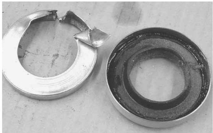
2) After machining-open the original seal, the metal "sleeve" (on the right) will be kept.
