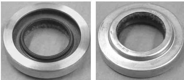
5 & 6) Aluminum bushing and seal, pressed into steel "sleeve." Felt "washer" helps keep road dust from reaching inner seal. Once installed in car, the new portion of the seal is totally concealed within the original steel shell.
