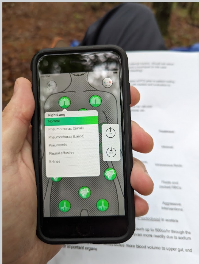
Figure 2. The “Remote” device (iPhone™) may be used to trigger the display of normal or pathologic cine loops.
