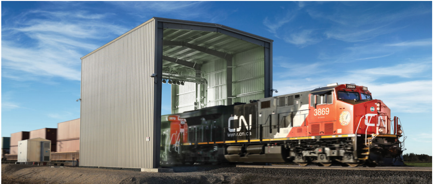
Automated inspection portals with ultra-high-definition panoramic cameras and infrared lighting capture a 360° view of a train as it travels at track speed, allowing the detection of many defects not visible to the human eye. CN photo
