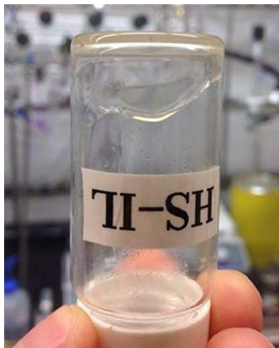
Figure 1. A porous ionic liquids composed of functionalized hollow silica nanospheres.
