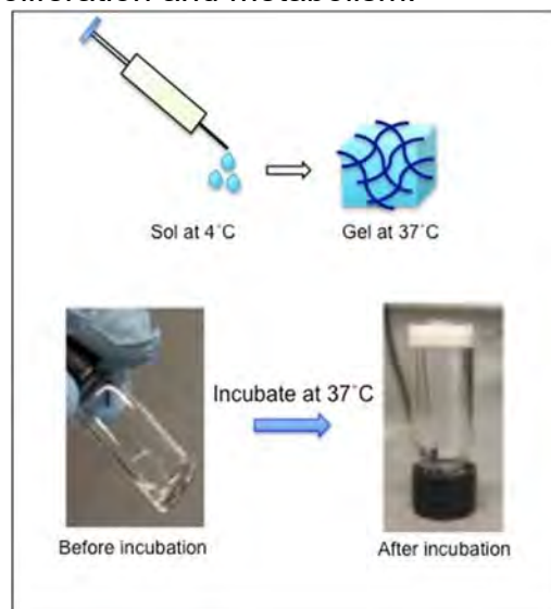
Figure 1. Schematic of gel formation; EC exists as solution (sol) at lower temperature and solid gel at 37°C. The approach combines syringeability of sol and in situ gelling properties of gel. Lower panel: Inversion test showing sol-gel transition using EC in 1x PBS at pH 7.4.
