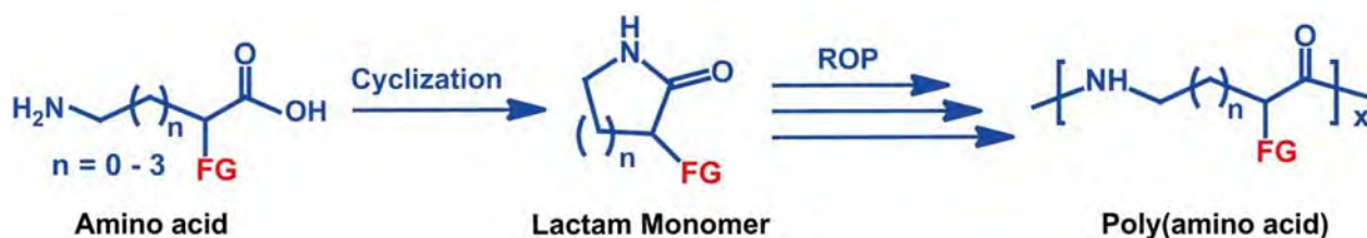
Figure 1. Ring-opening polymerization of lactam monomer for the synthesis of poly(amino acid).
