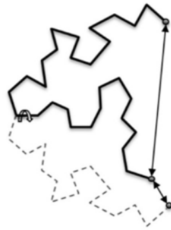
Illustration of the reduction in the end-to-end separation of polymer chain ends achieved by altering the conformation about a single backbone bond.
