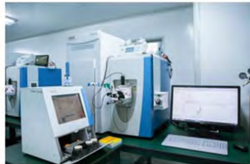
nano (High Performance Liquid Chromatography) HPLC – (Electronic Spray Ionization) ESI – Tandem Mass Spectroscopy (MS/MS) 11
