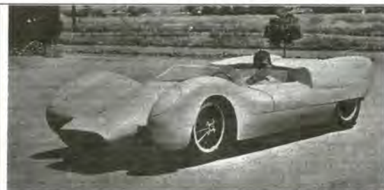
DESIGNER Bud Hull peers across wraparound windshield of his Dolphin America. Removable fender panels cover the headlights.
