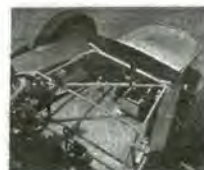
REMOVING front end of body reveals the leg opens for driver and passenger. The battery can be relocated to suit.
