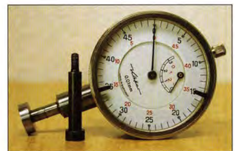
Dial indicator with tips for splitcase housings (8mm, mounted) and tunnel housings (20mm, foreground). Instrument dial rotates to zero-set.
