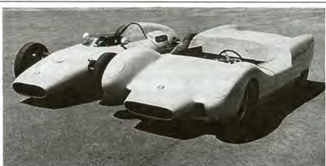
The Dolphin America (right) has a track four inches wider than the Junior from which it was derived, and carries an FIA passenger's seat which is as comfortable as the driver's.
