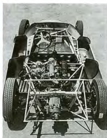
The independent rear suspension features an A-arm at the bottom and a simple tubular strut at the top end of a magnesium hub carrier. Both upper and lower arms are threaded for camber adjustment, and two long parallel radius rods locate the hubs and control toe-in.
