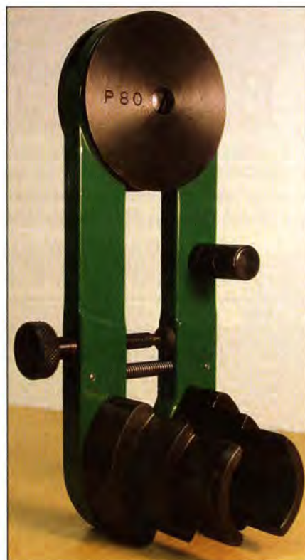
P 80, Porsche's own backlash tool, introduced in the early 1960s. Its longer jaws were better suited for tunnel-style housings.
