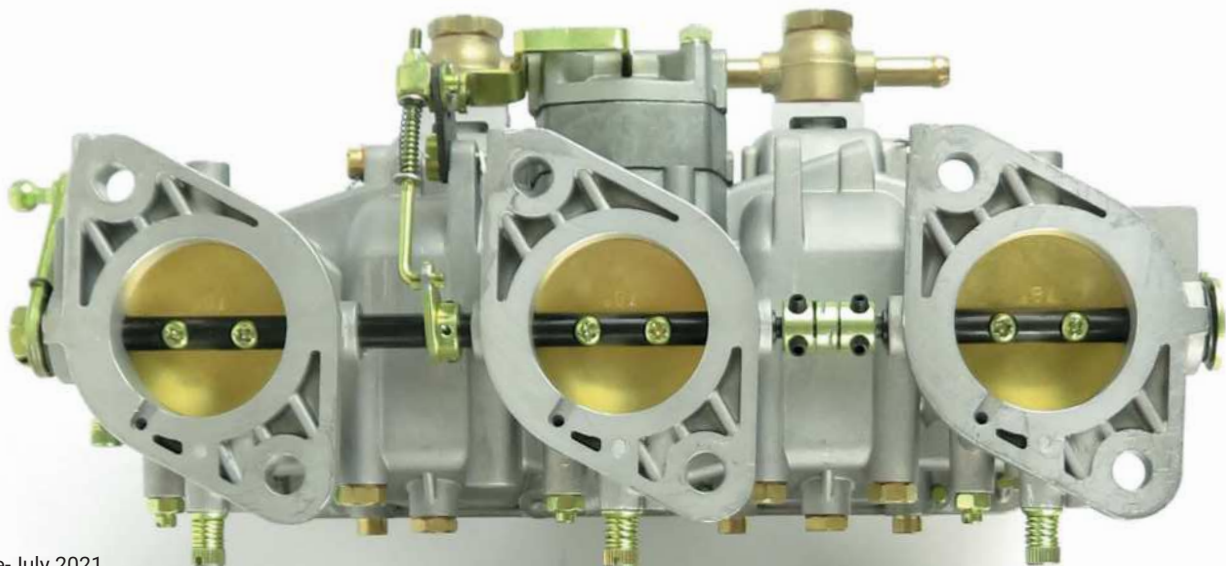
Below A single bank of Weber 40IDA3C carburetors for classic Porsche applications
