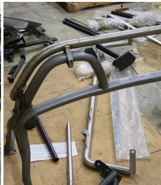
Left: Boxster roll bar extension turns the largely cosmetic hoops into something altogether more useful by adding height and extra strength
