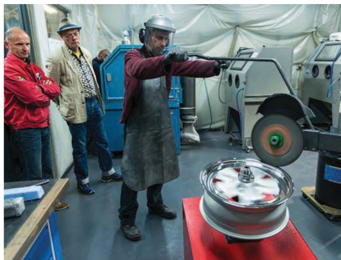
More specialist machinery, this time to polish the outer rim. Patrick Pugin insists on a 'clean air' environment, with extractors to remove any contamination
