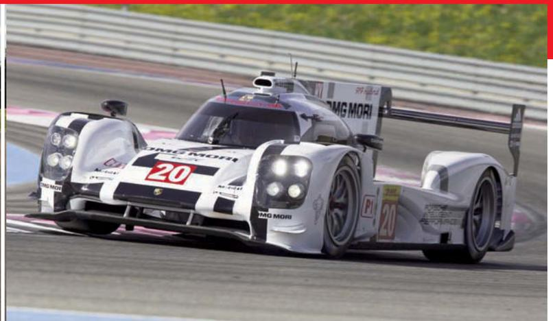
history and purpose built to dominate at Le Mans, Porsche describes the 919 as its "fastest ever research laboratory". The LMP1 Class racer runs a turbocharged 2.0-litre V4 petrol engine along with lithium-ion hybrid power and an advanced energy recovery system.
