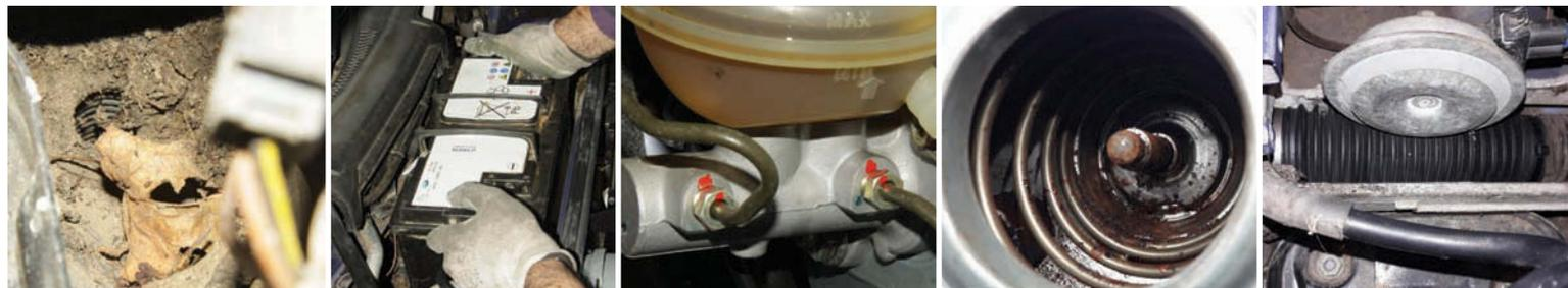
With 996's plenum-chamber cover removed, and then the battery, it was easy to see the composted leaves blocking the all-important drain holes. Red paint on hydraulic unions suggested servo was the original, superseded back in the day by one with an improved actuating-rod gaiter. Inside of old servo shows obvious evidence of corrosion
