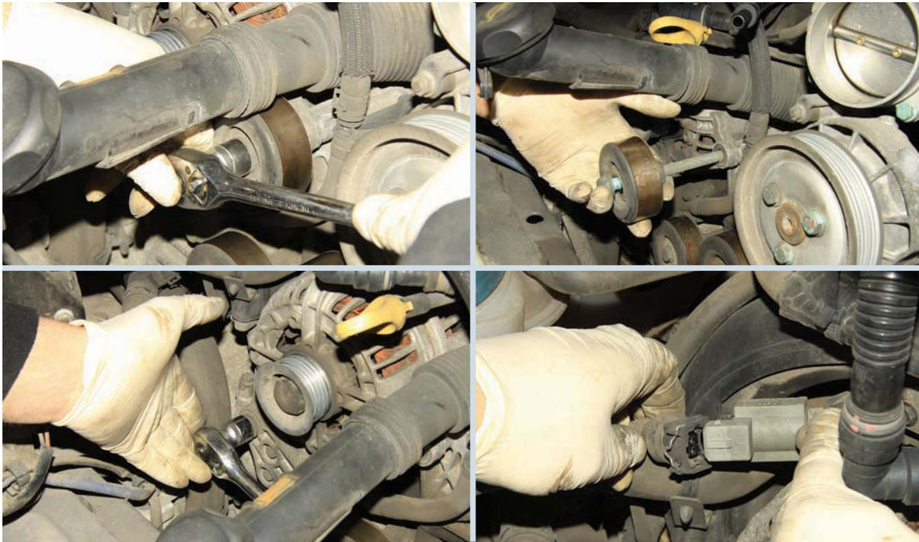
Once the auxiliary drive-belt is out of the way, undo first the long screw securing both the uppermost roller and one side of the alternator, and then the similar screw on the other side of the casing. Detach this electrical connection, too (below, near left)
