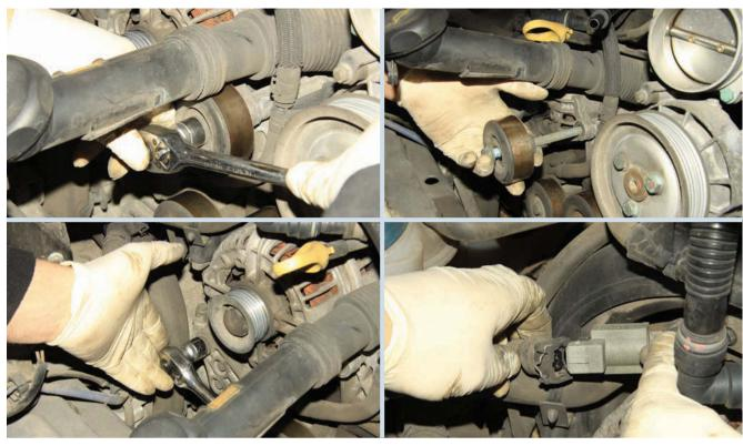
Once the auxiliary drive-belt is out of the way, undo first the long screw securing both the uppermost roller and one side of the alternator, and then the similar screw on the other side of the casing. Detach this electrical connection, too (below, near left)
