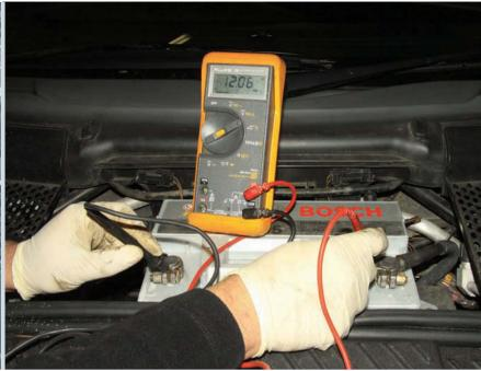
disconnect the battery before starting work on any vehicle's electrical system, and particularly so when dealing with the alternator. The latter's main output lead is by definition connected directly to the accumulator's positive terminal, and if while still live it touches any part of the adjacent metalwork, you will immediately have a pretty spectacular firework display – and quite possibly even a fire.
