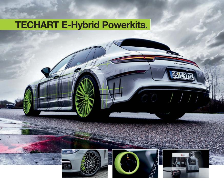
The TECHART TECHTRONIC engine powerkit for the Panamera Turbo S E-Hybrid boosts the standard combined power from 680 hp to 770 hp. The combined torque increases from max. 850 Nm to breathtaking 980 Nm.
