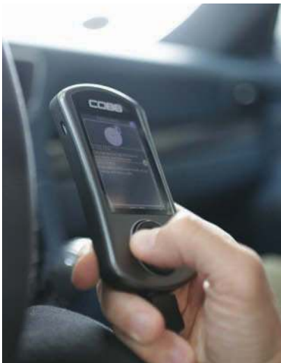
Hand held remote COBB ecu map and software controls everything from power stages to the speed of the PDK shift
