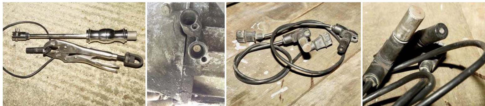
Combined self-grip pliers and slide hammer made pleasingly short work of extracting BMW engine's speed sensor, and later the identical reference sensor, but the former device left behind in the torque-converter housing its steel casing. That, and various other problems, could mean engine and transmission have to come out. Horton was hoping to use spare brand-new sensors bought for the red 924S (see previous page), but sadly their leads are far too short for the E28. Back to the drawing-board, then...
