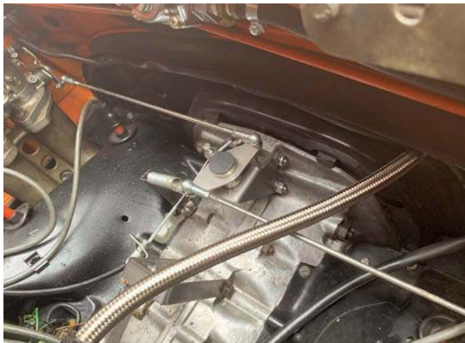
Above left and right: CSP bell-crank linkage has done wonders for the feel of the throttle pedal; a visit to Williams-Crawford sorted out the front-end suspension alignment
