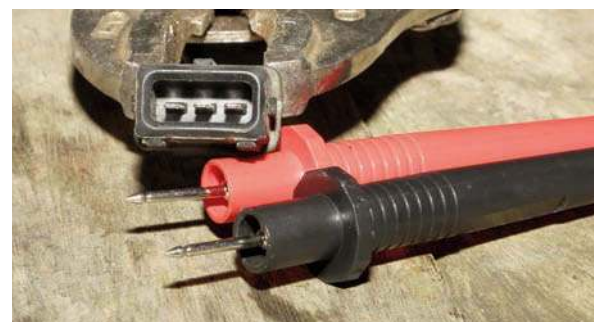
With sensor plug orientated as here, check resistance between first the left-hand terminal and the middle one, and then between left and right. BMW's were decisively open circuit, ie unserviceable
