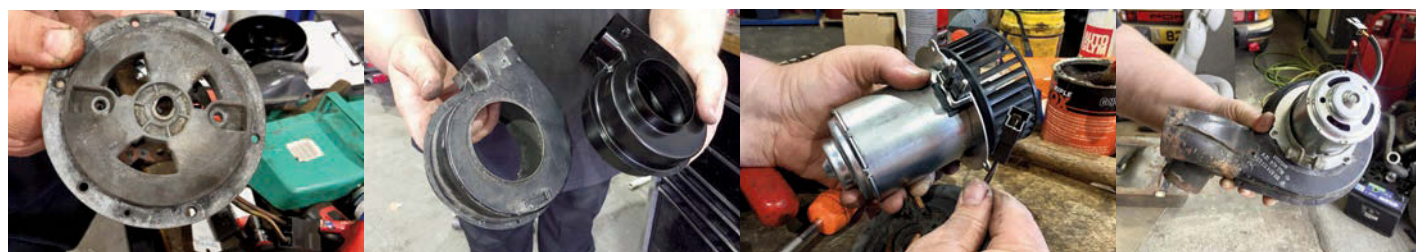
911SC's heater blower was completely worn out (far left), and as a result making an appalling racket when operating. Replacement motors are available from Porsche, but less expensive after-market units appear to be designed for cars up to and including the 964, and as a result require a few simple modifications
