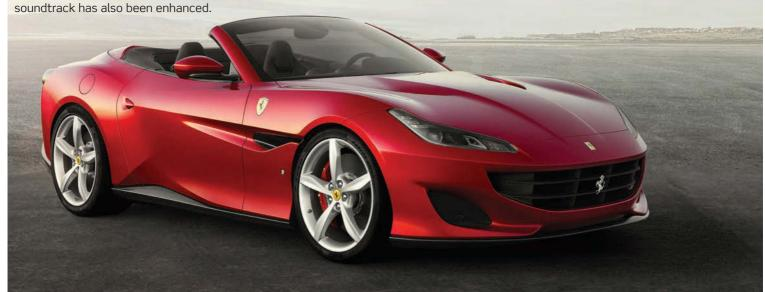
The chassis is all-new, featuring lower weight than the California T and increased torsional rigidity. Ferrari's third-generation electronic rear differential (E-Diff3) is adopted, while the Portofino also becomes Ferrari's first GT to be fitted with electric power steering, enabling a faster steering ratio. The damping system has been uprated, too, reducing roll and improving bump absorption.
