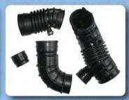
TS and V6 intake rubber pipes are a specialty. It is a part that often needs to be replaced on cars getting on for 20 years old and as we have had them made in large quantities, should have them available for the next 20 years! 3.0 and 3.2 intake runner pipes also made exclusively for us.
