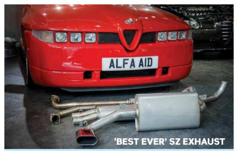
Berkshire-based Alfa Aid has produced "the best sounding SZ in the world" with a new exhaust system for the Alfa Romeo SZ ES30. Made from 304-grade stainless steel with a high chromium and nickel content, the system features tig-welded joints, CNC bends and flexible joints in stainless steel. All the original mounting points are used and it fits standard SZ manifolds.
