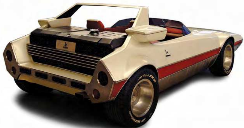
ABOVE & BELOW: The Runabout concept used the transverse engine/gearbox introduced in the Autobianchi Primula in 1964, placed behind the seats
