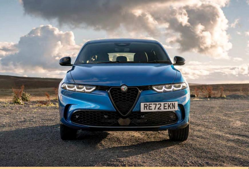
for my first drive on UK roads (I'm not going to count a quick hoof up the hill at Goodwood back in June). The only power option at launch in the UK is the Hybrid 160 (in other markets it's offered in Hybrid 130, diesel and pure petrol forms). There's a 1.5-litre turbocharged petrol engine mated to a small 48-volt electric motor (15kW of power and 55Nm of torque), providing 16ohp of power in total.
