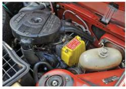
inline 'four', designed by none other than Aurelio Lampredi, the mastermind behind some of Ferrari's greatest competition engines. High-revving and over-square, the compact unit provided the 128 with the kind of zesty performance that didn't compute with its boxy lines.
