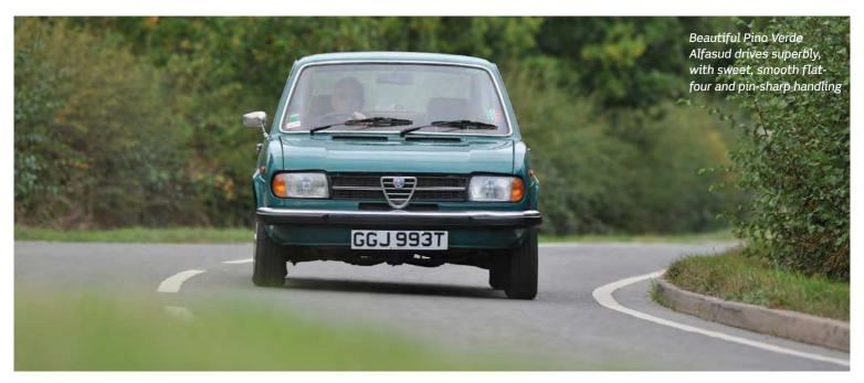
correct 145-section Pirelli Cinturatos. But it's the direct rack-and-pinion steering, engaging and full of feedback, that gives you so much confidence to press on. And when you do, the car's light weight (822kg) and sophisticated chassis elicit the sort of body control that could show British sports cars of the day a clean pair of heels.
