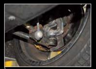
If front ball joints are creaking, investigate immediately. If they fail, you can lose a wheel Early 4Cs suffered from condensation and mouldy boots. Later versions have a boot lid liner
