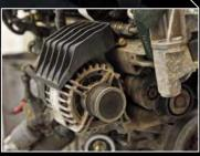
Alternators can suffer from water ingress, resulting in seizure or even the casings splitting in two
