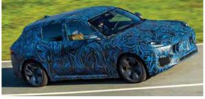
when they're specified – called Offroad. The driver can independently choose from two increased ride heights and one reduced, while the system automatically lowers the car further again once over about 80mph. The most basic Grecales will feature conventional steel springs with frequency selective damping and it will also be possible to order adaptive damping without air suspension, but our drive shows that the most
