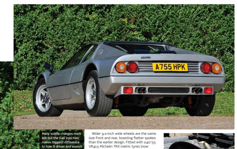
Wider 9.0-inch wide wheels are the same size front and rear, boasting flatter spokes than the earlier design. Fitted with 240/55 VR415 Michelin TRX metric tyres (now impossible to source), the result is a slightly wider track front and rear. This all translates to a more planted feel around corners, with less uncertainty on turn-in, more grip through each apex and a flatter cornering stance. The steering is still weighty, though, and the BBi is clearly more prone to following ruts in the road.
