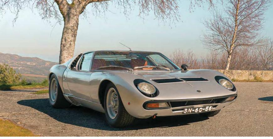
complex, yet tuneful. The clutch is heavy, for sure, but it's very progressive and doesn't need many revs on take-off. Peak torque comes at a rather high 5750rpm, but the SV weighs only 1293kg so it never feels slow.
