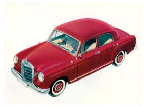
**Above:** Check the sills and front wings, both rust prone. condition and fitting a new one is a surprisingly big job involving several hours' labour. Otherwise check that the springs haven't sagged and that the rubber mountings blocks for the axle and trailing arms are all sound, as is the metal they attach to.
