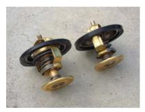
the open position, or the thermostat having been removed. Sometimes a faulty fan will also cause excess cooling – an electric fan that runs all the time, or a viscous coupling mounted oneon which the coupling has failed, meaning the fan turns all the time rather than being able to slip until the engine reaches temperature.
