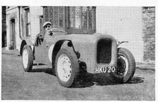
ANOTHER IN FIBRE GLASS: Amongst the widely variegated types of cars running in last Saturday's 750 MC Relay Race was W. D. Binns's Mk. V Buckler, fitted with resin-bonded glass body made by Versil Ltd., of Liver-sedge, Yorks.
